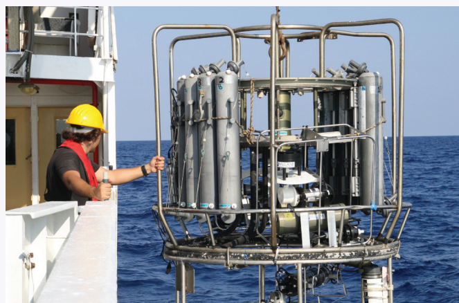
A CTD Rosette used for sampling deep sea water
